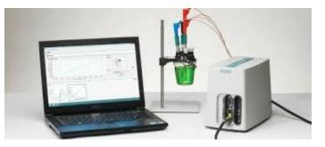
response analyser (FRA) designed for general purpose electrochemical measurements. Based on the workstation quite a number of new experiments can be performed.
